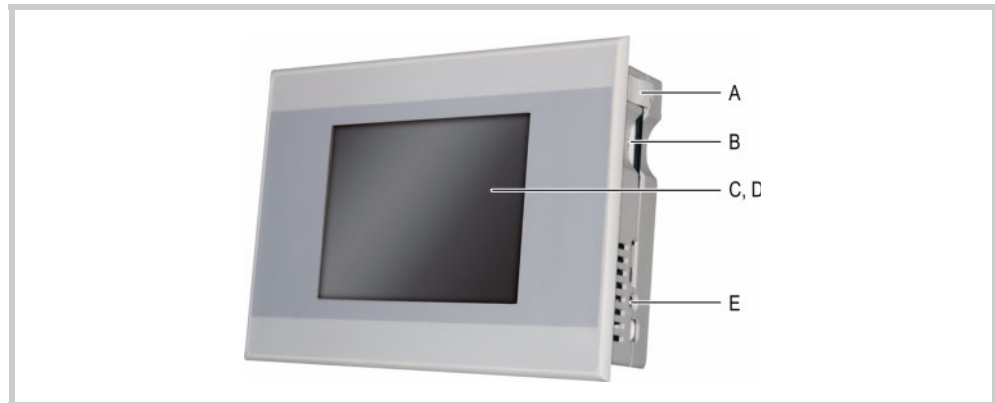
Fig. 2 Operating and indication elements
