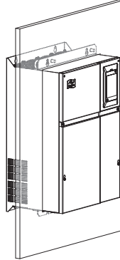
Figure 3-11 Embedded installation effect of the IS300 (sheet metal housing)
