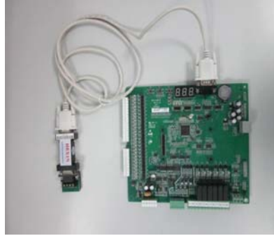
Figure 6-2 Parallel connection at the monitoring port
