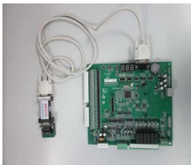
Figure 6-2 Parallel connection at the monitoring port
