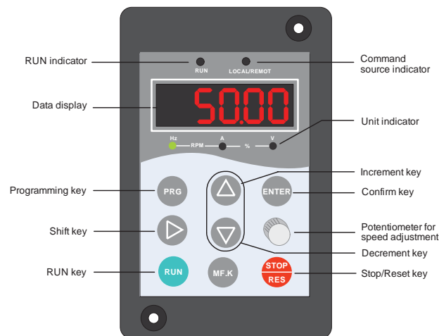
Figure 4-2 Diagram of the operation panel (with the potentiometer)
