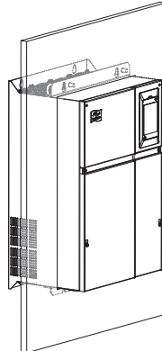
Figure 3-11 Embedded installation effect of the MD280 (sheet metal housing)
