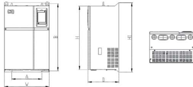
Schematic Diagram for Physical Dimensions and Mounting Dimensions of 18.5kW-90kW
