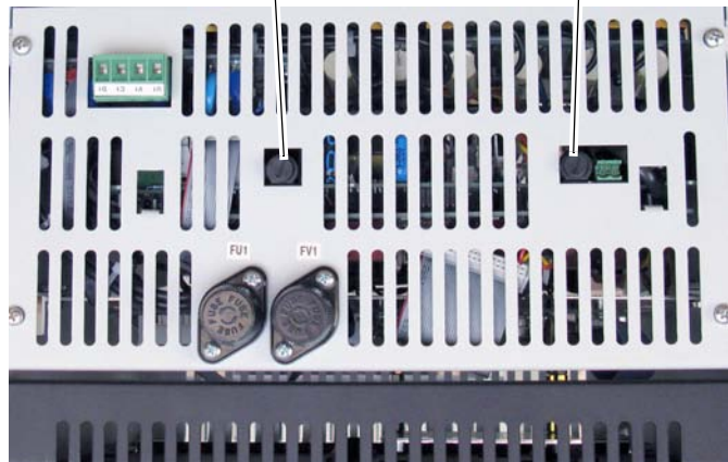
Figure 63 - Frame C Switching Power Supply Circuit Board Fuse Location
