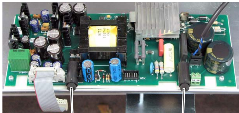
Figure 63 - Frame C Switching Power Supply Circuit Board Fuse Location
