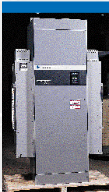
300 HP Custom NEMA Type 12 Drive with Dual Air Conditioners for Internally Mounted Drive Heatsink.
