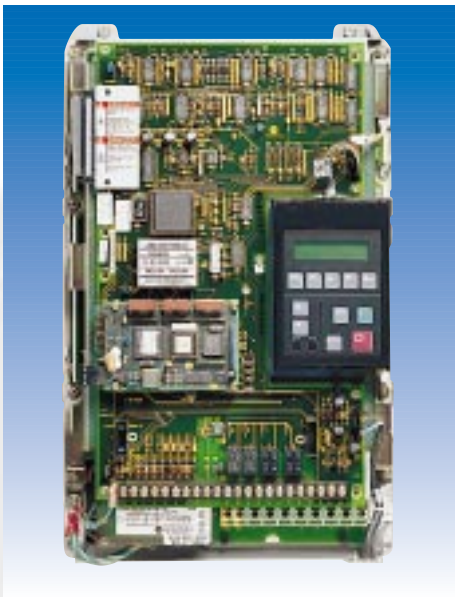
Standard 1336 PLUS Variable Frequency Drive with Programming Panel
