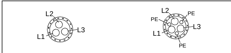
Figure A-2 Recommended motor cables.
